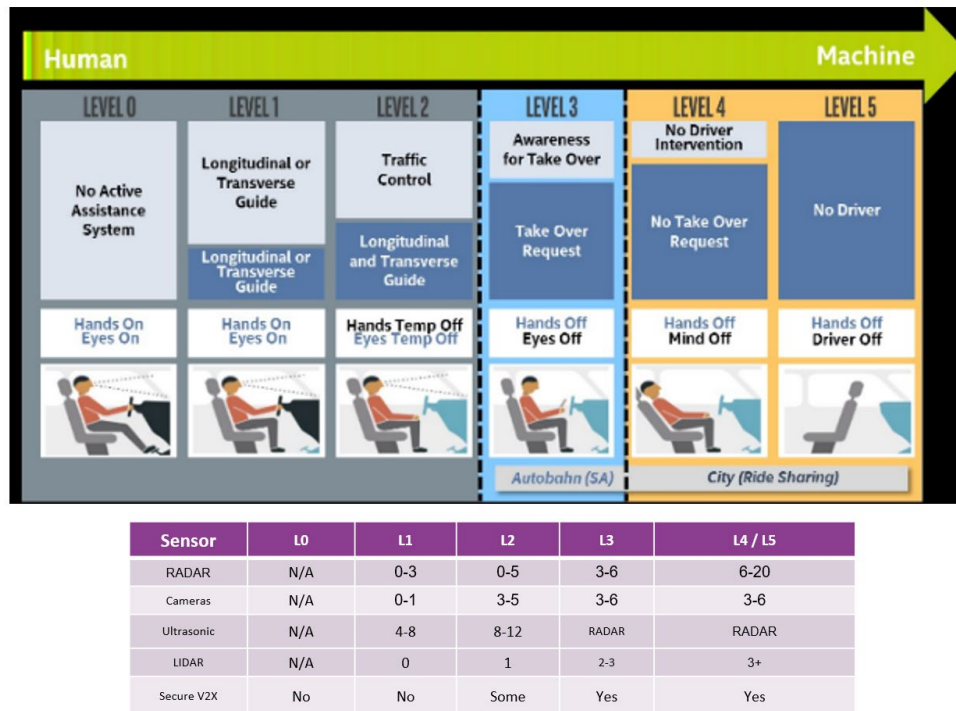
Figure 1. The need for human interaction and attention decreases at higher levels of driving automation.
