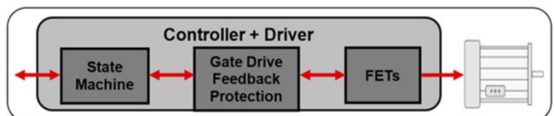
Shown is an intelligent integrated BLDC motor driver.
