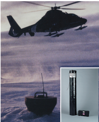
Converting to PulsesPlus battery packs reduced the size of a device that monitors the size and location of icebergs. The larger battery pack (left) used 380 D-size alkaline cells while the far more compact battery pack (right) used 32 lithium D-cells and 4 AA-sized hybrid layer capacitors (HLCs).
