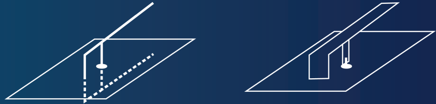
Figure 2: Inverted "F" Antenna evolution from the L-antenna by feeding the antenna at a more favorable impedance point (left); extruded version of Inverted F antenna to produced Planar Inverted F antenna or PIFA (right).
