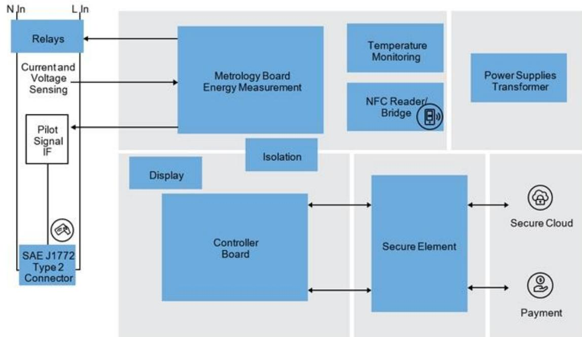
System-level view of an EVSE
