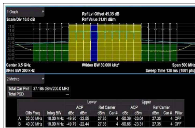
▲ Fig. 10 ACLR plot for Wolfspeed fully integrated PA with DPD linearization for 10C x 20 MHz LTE signal (200 MHz IBW).
