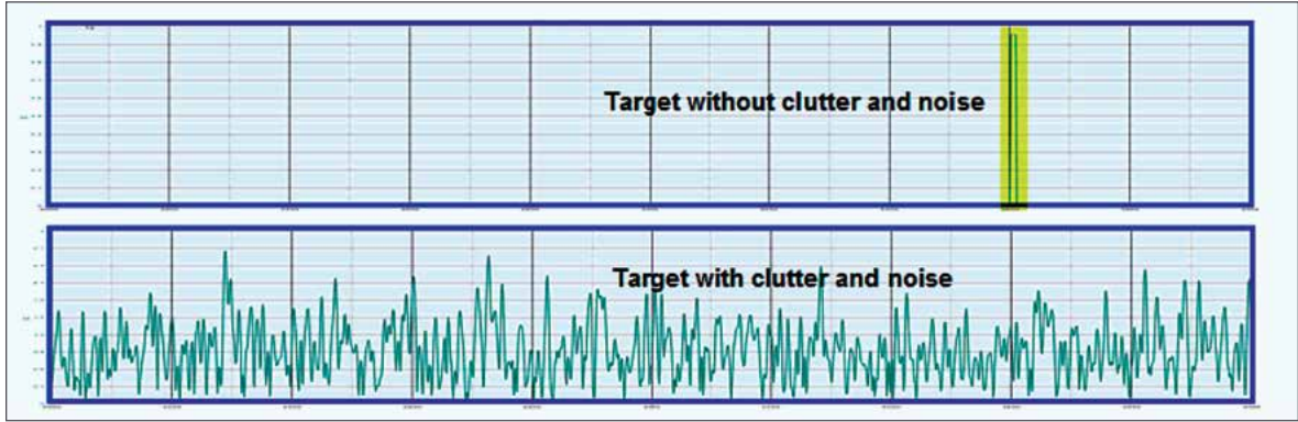
Figure 4.5. Target signal hidden by heavily cluttered environment
