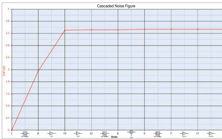
Figure 3.8b. Noise-figure budget analysis of receiver front end
