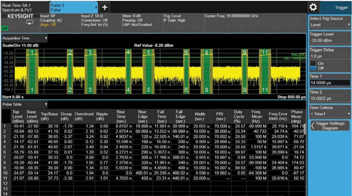
Figure 22.24. The N9067C embedded pulse application can display numerous pulse statistics, simplifying the characterization of dense pulse environments.
