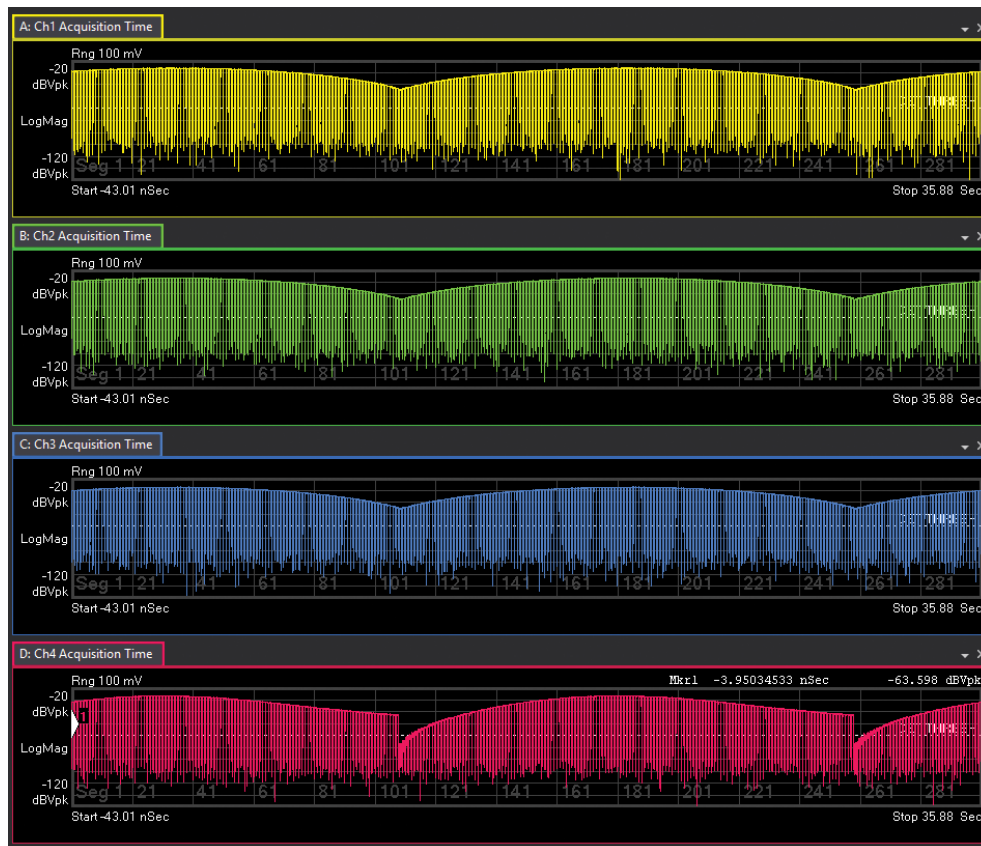
Figure 17.21. Segmented capture across four channels
