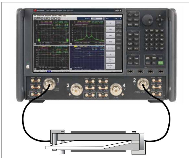
Figure 15.7. Resonant cavity method with network analyzer
