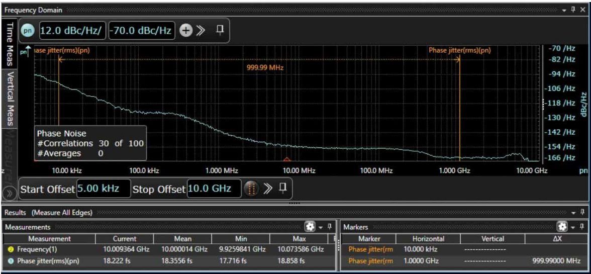
Figure 11.6. Infiniium Real-Time Oscilloscope phase noise interface.
