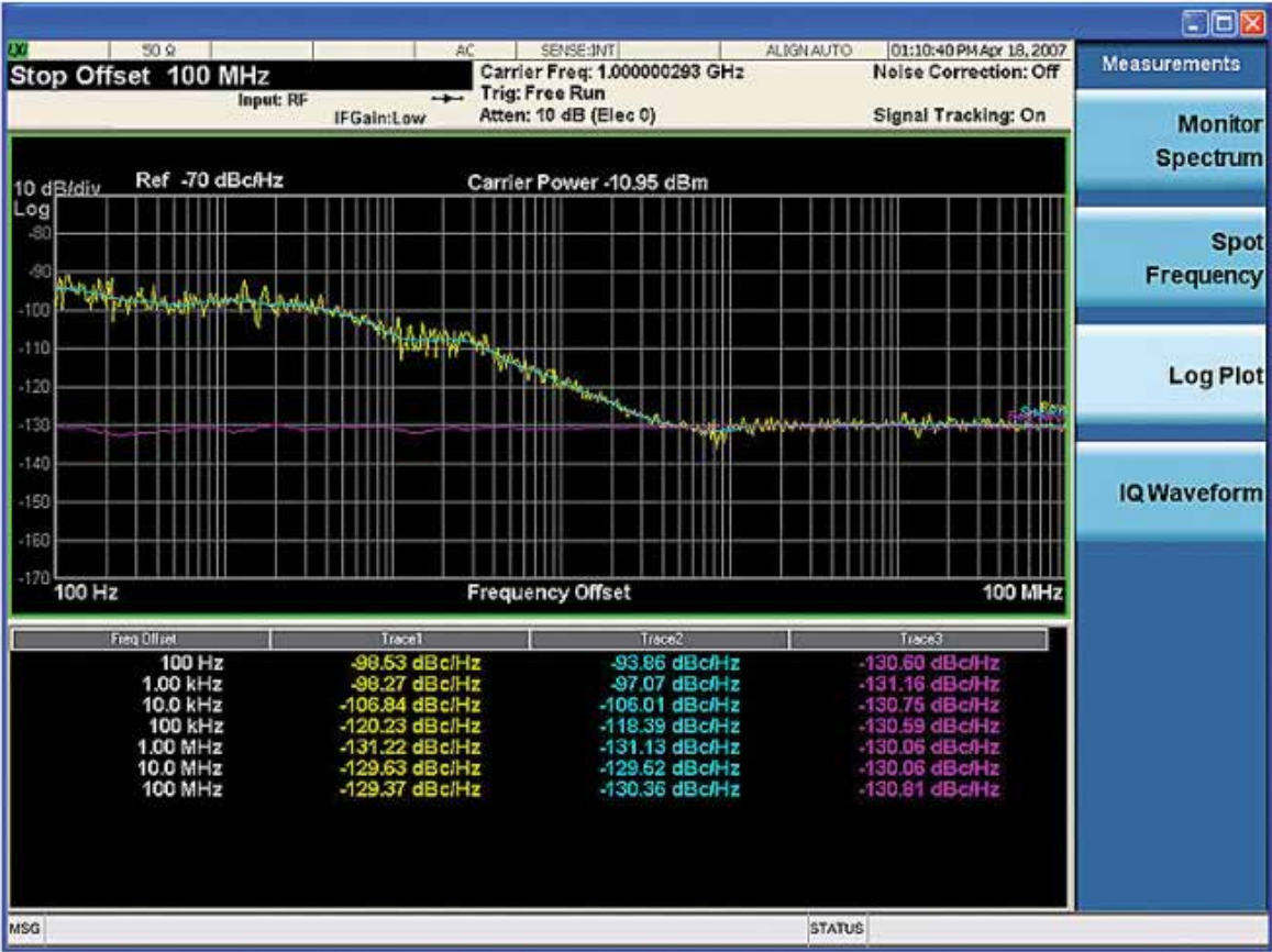
Figure 11.7. Keysight X-Series signal analyzers phase noise measurement application.
