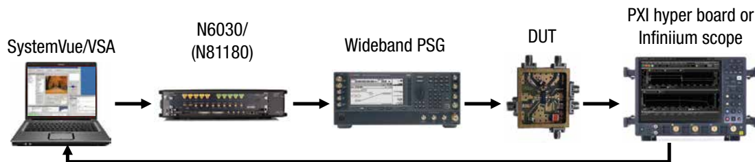
Figure 7.10. Test setup for wideband signal generation.
