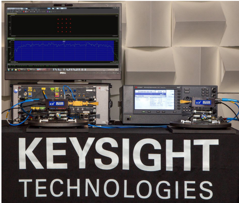
Figure 11. 16 QAM OTA measurements performed at 144 GHz with G-band VDI converters, 10 GHz occupied bandwidth
